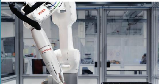
↑ ItemPiQ is designed to do order fulfilment fast - up to 1,000 picks per hour.
